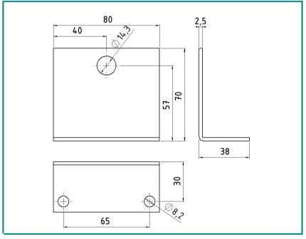
The wall mounting bracket with the corresponding housing nut assures the secure mounting of the pressure regulator FHR 3 and FHR 4.
